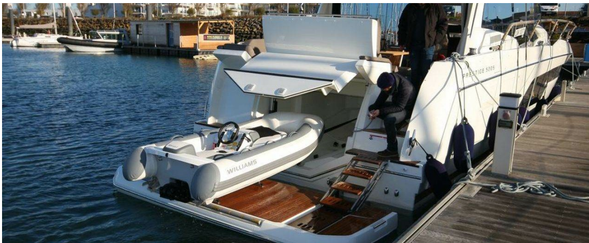
Transom garage for tender with electrically-opening door
