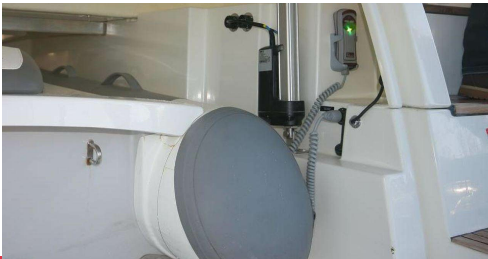
Transom garage for tender with electrically-opening door
