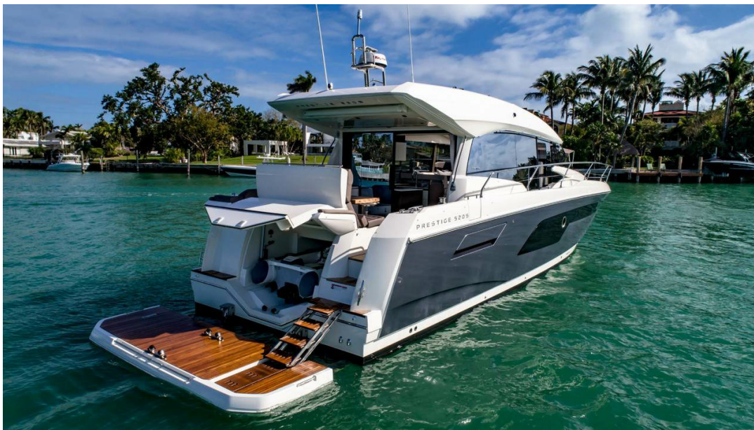
Large hydraulic platform
